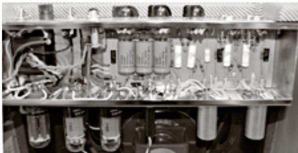
just grounded one leg of the 6.3V to the chassis, (to use it as one side of the filament), and ran one wire to the other side of the filaments. We use the same wire routing, the same construction techniques with brass eyelets, all carbon comp Allen Bradley resistors, Carling switches, and the tube sockets are NOS made for the military in 1952.
